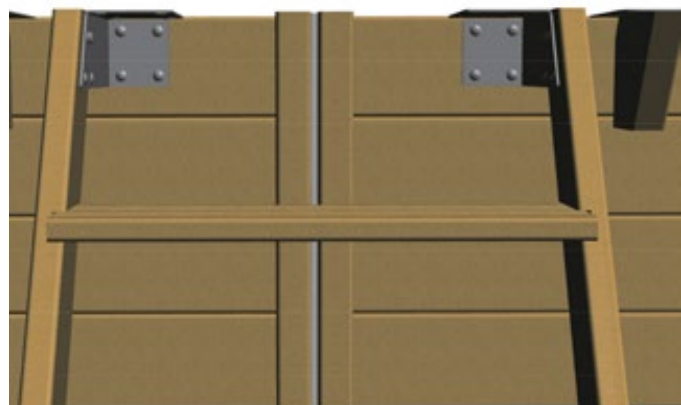
Figure 17 – Fastening the access ladder to the pool wall
